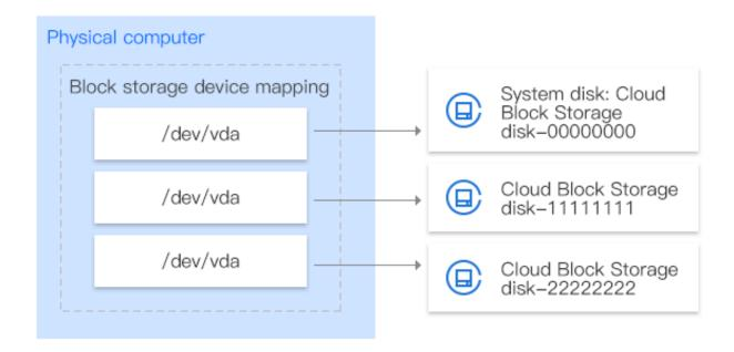
This figure shows how CBS maps the block storage device to the CVM and maps /dev/vda' to the system disk, and how it maps the two data disks to '/dev/vdb and /dev/vdc' respectively.
